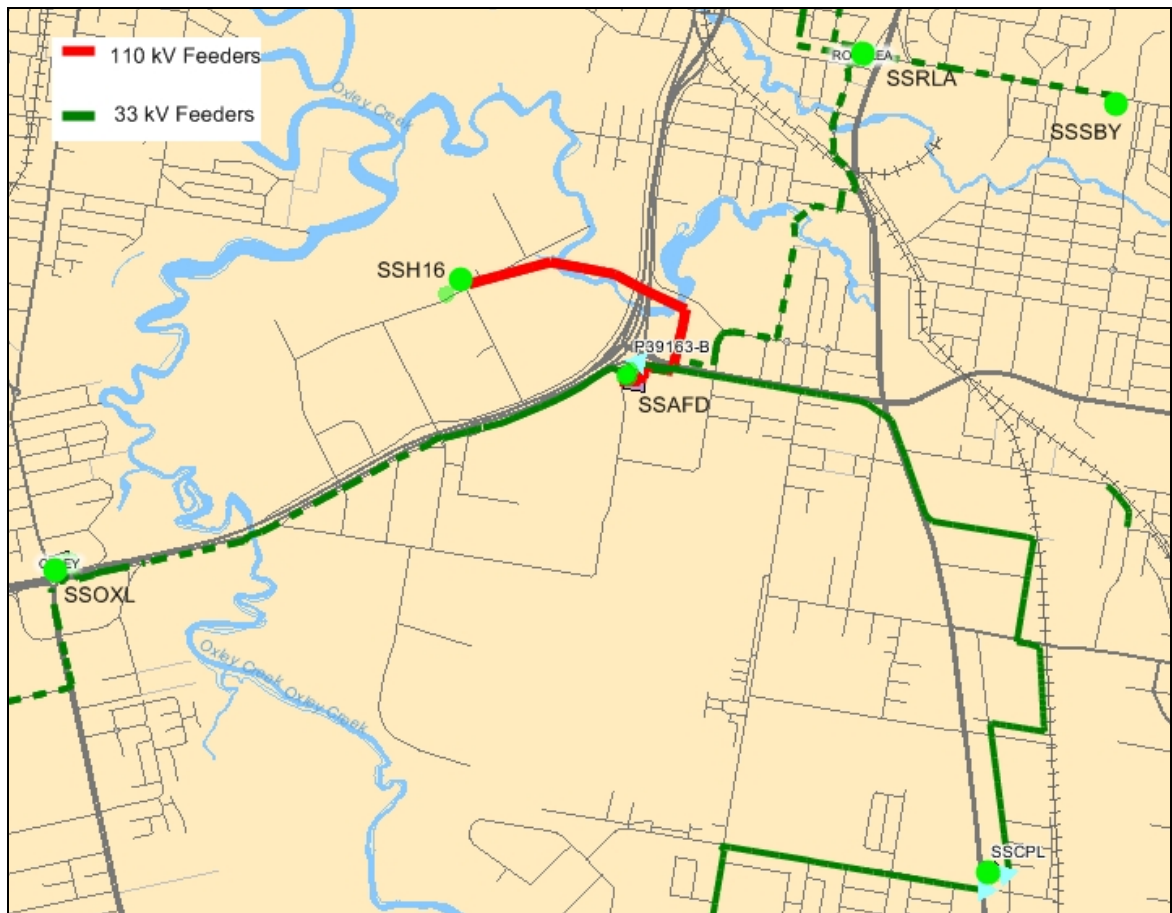
Figure 1: Existing Network Arrangement (Geographic View)
