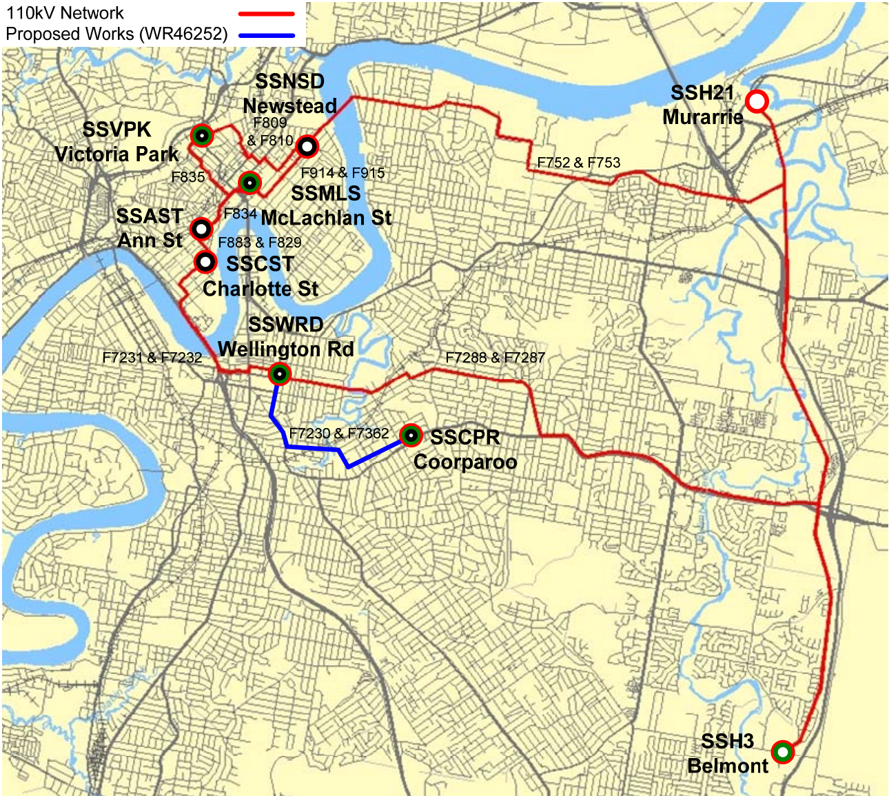
Figure 11: Proposed 110 kV Network Arrangement (Geographic View)
