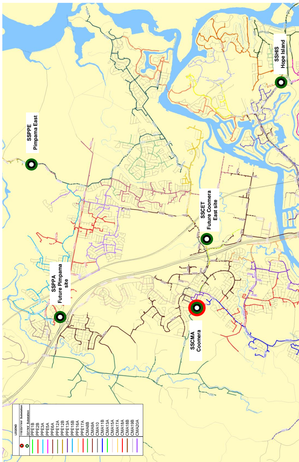
Figure 3: Existing 11kV network arrangement (geographic view)
