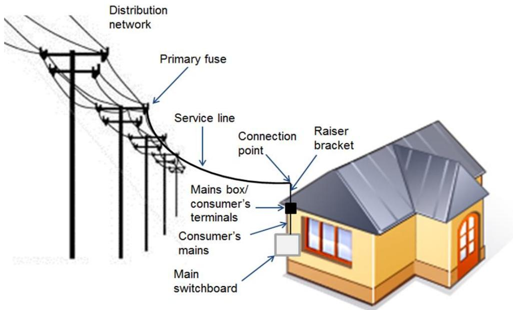
For premises located in an area with underground electricity supply, the connection typically involves the customer's consumer mains connecting into a connection point in an Energex-owned distribution service pillar. The customer is then responsible for the consumer's mains. This is illustrated in the following diagram.
