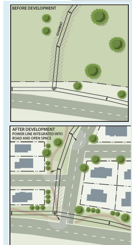
**Figure 3: Subdivision design is crucial in the protection and performance of both sub-transmission and distribution powerlines. The above image shows successful easement integration, where the line is located in open space and the road reserve. Good design outcomes can lead to successful and sustainable easement co-use.**
