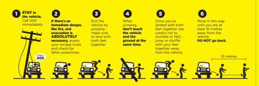
We recommend that operators of machinery practise this jump / shuffle technique on a regular basis.
