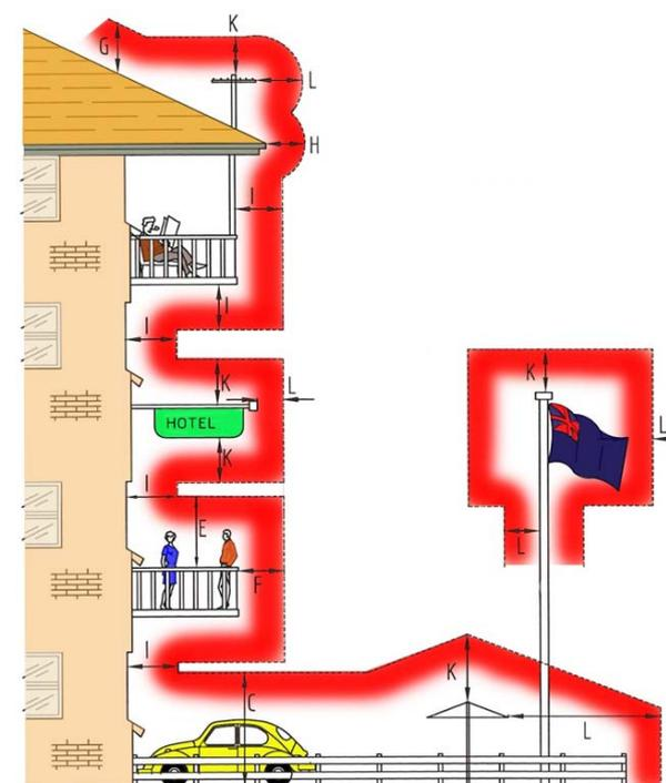
Where the Electricity Entity has identified a breach of statutory clearance resulting from erection of a building or structure, the statutory breach will be reportable to the Electrical Safety Office as a Dangerous Electrical Event and any costs incurred in subsequent remedial work to achieve required statutory clearances may be recovered from the person or company who caused the breach of statutory clearance.
