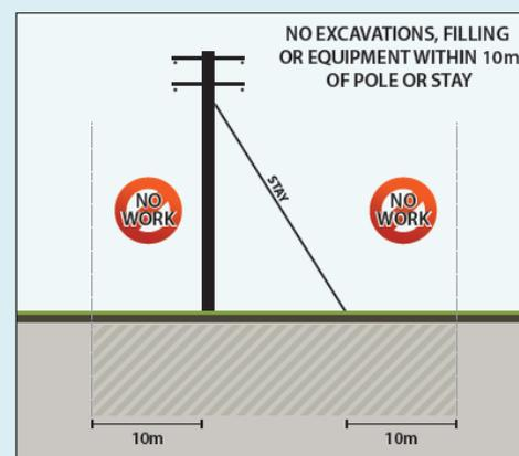
'No civil works zones' of 10 metres are established around our transmission and distribution structures to ensure the structural integrity of the asset is maintained. Works are allowed within these zones if appropriate measures are taken to support the structure during and after the completion of works. These measures must be verified with an assessment by us.
