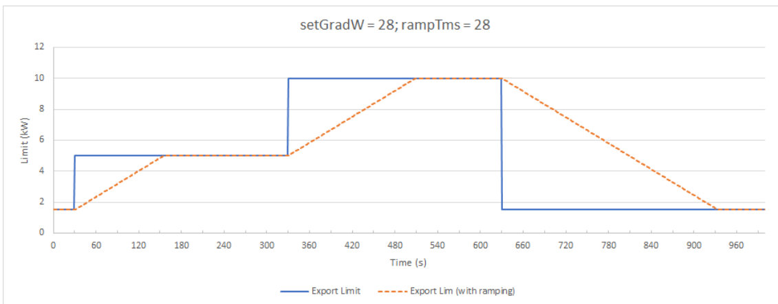
Figure 6: Example where rampTms and setGradW are the same, or rampTms not set.
