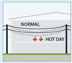
Powerline sag is a reaction to climate temperatures and operating conditions. Filling under a line can impact on statutory clearances to the ground if final clearance levels do not allow for any 'sag'.
