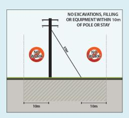
'No civil works zones' of 10 metres are established around our transmission and distribution structures to ensure the structural integrity of the asset is maintained. Works are allowed within these zones if appropriate measures are taken to support the structure during and after the completion of works. These measures must be verified with an assessment by us.
