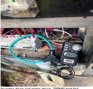
Inverter does not ramp down -DRM0 test fail
