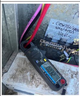
Inverter ramps down in DRM0 test
