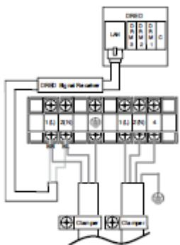
※ Make use of the wires connected with O-ring.
