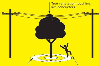
If tree foliage is touching the overhead conductors, transferring voltage to the base of the tree, hazardous voltages may also be present for some distance around the base of the tree at ground level. This area is called the Surface Voltage Gradient area This person could be affected by a value of step potential.
