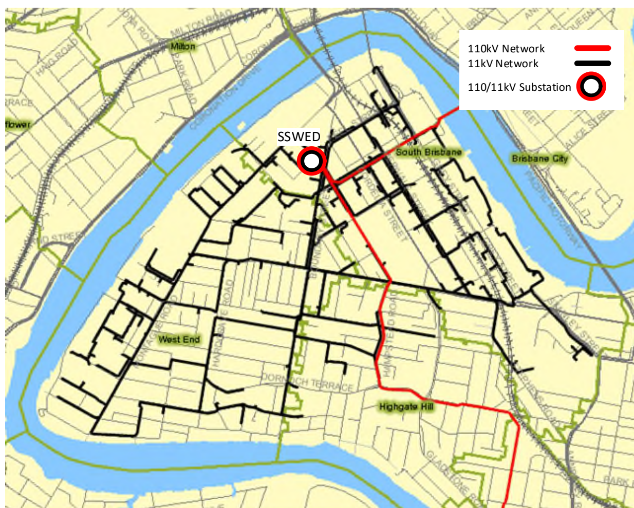
Figure 1: Existing SSWED network arrangement (geographic view)
